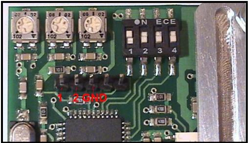
There's an option to connect two safety limit switches to the controller. The factory programming terminal has two pins(pin 1. and 2.), which are inputs and used to disable the running of the controller to one-one direction.
