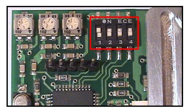
The DIP switch contains 4 on/off switches. The meaning of the switches follows:
