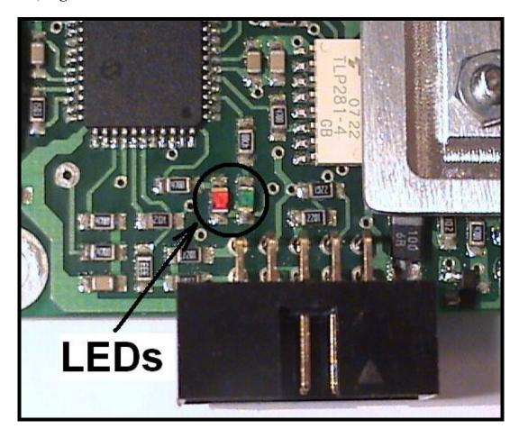
There are two LEDs on the board, one green and one red LED.
