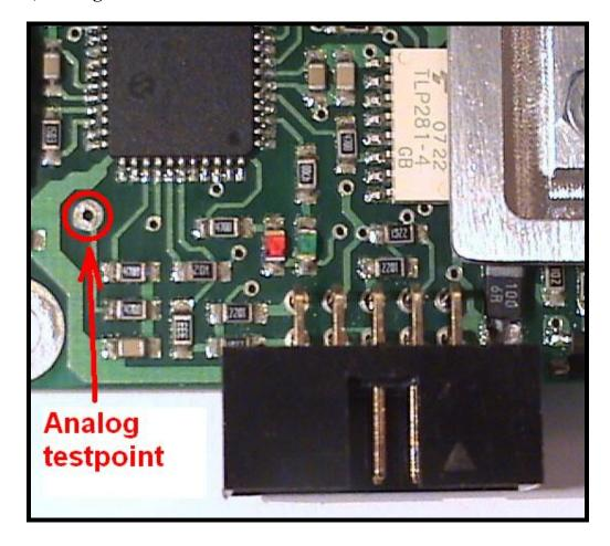
There's a testpoint on the board with an analog output, the analog signal is proportional to the servo error.
