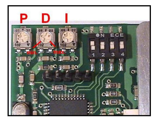
There are 3 potentiometers placed onto the board.
